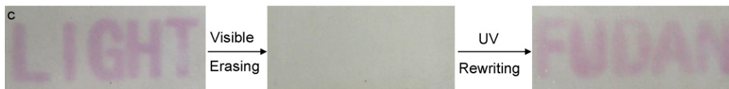
Fig. 4. (a) Time dependence of the absorption at 550 nm of dispersed SP-MnPS 3 nanoparticles (triangle mark, [c] SP = 2.0 × 10 -4 mol/L) and of nanofilm (square mark), respectively, under irradiation (365 nm, filled mark) and bleaching (550 nm, empty mark). (b) Cycles of colouration and bleaching on the nanofilm. (c) Photo-rewritable imaging on the nanofilm of SP-MnPS 3 by using UV (365 nm, hand-held lamp) and visible light (>500 nm). The violet regions represent the parts irradiated with UV light.
